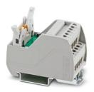
VARIOFACE module, with screw connection and flat-ribbon cable connector, for mounting on NS 35 rails, with pin strip and short and long locking latches for socket strips, 10-pos.
