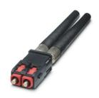
FO connectors, degree of protection: IP20, number of positions: 2, MM, material: Plastic, connection method: mechanical splice, cable outlet: straight, color: black, Ethernet
