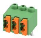
PCB terminal block, nominal current: 4 A, rated voltage (III/2): 250 V, nominal cross section: 0.5 mm<sup>2</sup>, number of potentials: 3, number of rows: 1, number of positions per row: 3, product range: FK-MPT 0,5/..-H, pitch: 3.5 mm, connection method: Push-in spring connection, mounting: Wave soldering, conductor/PCB connection direction: 0 °, color: green, Pin layout: Linear pinning, Solder pin [P]: 4 mm, number of solder pins per potential: 1, type of packaging: packed in cardboard
