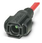
Device connector front mounting, Range of articles: SUNCLIX, housing material: PPE, color: black, number of positions: 1, min. conductor cross section: 2.5 mm<sup>2</sup>, rated voltage: 1000 V DC, rated current: 27 A, Connection method: Crimp, Contact connection type: Pin, cable length: 120
