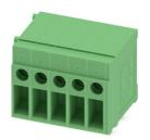
PCB terminal block, nominal current: 32 A, rated voltage (III/2): 320 V, nominal cross section: 4 mm², number of potentials: 5, number of rows: 1, number of positions per row: 5, product range: FRONT 4-H, pitch: 6.35 mm, connection method: Front screw connection, mounting: Wave soldering, conductor/PCB connection direction: 0 °, color: green, Pin layout: Linear pinning, Solder pin [P]: 5 mm, number of solder pins per potential: 2, type of packaging: packed in cardboard
