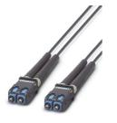
Assembled FO cable, breakout cable, 980/1000  $\mu m$  polymer fiber, SC-RJ/IP20 to SC-RJ/IP20, for installation inside control cabinets, the cable is suitable for UV-protected outdoor use, length: 2 m
