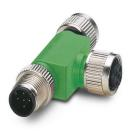
T distributor, 5-position, Plug straight M12, coding: A, on Socket straight M12, coding: A and Socket straight M12, coding: A, Parallel distributor
