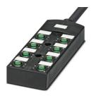
Distributor box, application: Standard, connection method: M12-SPEEDCON-socket Metal, number of slots: 8, number of positions: 5, coding: A, slot assignment: Double, status display: Yes, pnp; master cable connection: Fixed connection 180°, PUR/PVC, cable length: 10 m, shielding: no
