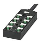
Distributor box, application: Standard, connection method: M12-SPEEDCON-socket Metal, number of slots: 8, number of positions: 5, coding: A, slot assignment: Double, status display: Yes, pnp; master cable connection: Fixed connection 180°, PUR/PVC, cable length: 5 m, shielding: no
