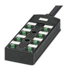
Distributor box, application: Standard, connection method: M12-SPEEDCON-socket Metal, number of slots: 8, number of positions: 4, coding: A, slot assignment: single, status display: Yes, pnp; master cable connection: Fixed connection 180°, PUR/PVC, cable length: 10 m, shielding: no
