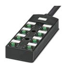
Distributor box, application: Standard, connection method: M12-SPEEDCON-socket Metal, number of slots: 8, number of positions: 4, coding: A, slot assignment: single, status display: Yes, pnp; master cable connection: Fixed connection 180°, PUR/PVC, cable length: 5 m, shielding: no
