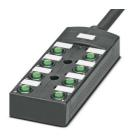
Distributor box, application: Standard, connection method: M12-SPEEDCON-socket Metal, number of slots: 8, number of positions: 5, coding: A, slot assignment: Double, status display: No, Universal; master cable connection: Fixed connection 180°, PUR/PVC, cable length: 10 m, shielding: no
