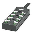
Distributor box, application: Standard, connection method: M12-SPEEDCON-socket Metal, number of slots: 8, number of positions: 5, coding: A, slot assignment: Double, status display: No, Universal; master cable connection: Fixed connection 180°, PUR/PVC, cable length: 5 m, shielding: no
