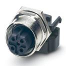
Sensor/Actuator flush-type socket, 5-pos., M12, B-coded, rear/screw mounting with M12 thread, with straight solder connection
