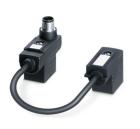
Double valve connector adapter, Universal, 4-position, PUR/PVC, black RAL 9005, Plug straight M12 SPEEDCON, coding: A, on Valve connector BI (11 mm), with 1 LED, Wiring: Z diode and Valve connector BI (11 mm), with 1 LED, Wiring: Z diode, valve connector spacing: 0.2 m
