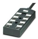
Distributor box, application: External areas, connection method: M12 socket Metal, number of slots: 8, number of positions: 5, coding: A, slot assignment: Double, status display: No, Universal; master cable connection: Fixed connection 180°, PUR/PVC, cable length: 5 m, shielding: no
