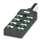
Distributor box, application: Standard, connection method: M12-SPEEDCON-socket Plastic, number of slots: 8, number of positions: 5, coding: A, slot assignment: Double, status display: Yes, pnp; master cable connection: Fixed connection 180°, PUR/PVC, cable length: 10 m, shielding: no
