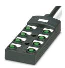
Distributor box, application: Standard, connection method: M12-SPEEDCON-socket Plastic, number of slots: 8, number of positions: 5, coding: A, slot assignment: Double, status display: Yes, pnp; master cable connection: Fixed connection 180°, PUR/PVC, cable length: 5 m, shielding: no
