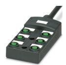
Distributor box, application: Standard, connection method: M12-SPEEDCON-socket Plastic, number of slots: 6, number of positions: 4, coding: A, slot assignment: single, status display: Yes, pnp; master cable connection: Fixed connection 180°, PUR/PVC, cable length: 10 m, shielding: no
