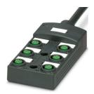
Distributor box, application: Standard, connection method: M12-SPEEDCON-socket Plastic, number of slots: 6, number of positions: 5, coding: A, slot assignment: Double, status display: No, Universal; master cable connection: Fixed connection 180°, PUR/PVC, cable length: 10 m, shielding: no
