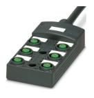
Distributor box, application: Standard, connection method: M12-SPEEDCON-socket Plastic, number of slots: 6, number of positions: 4, coding: A, slot assignment: single, status display: No, Universal; master cable connection: Fixed connection 180°, PUR/PVC, cable length: 10 m, shielding: no
