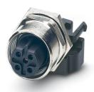
Sensor/actuator flush-type connector, socket, 5-pos., M12, shielded, B-coded, rear/screw mounting with M12 thread, with polarity protection, with straight solder connection
