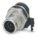
Device connector rear mounting, 8-position, Pin, angled, M12-SPEEDCON, coding: A, Rear mounting, M12 x 1, Solder pins, Alternative product in accordance with RoHS II without Exemption 6c (Pb < 0.1 %) item no.: 1239642
