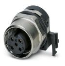
Device connector rear mounting, 5-position, Socket, angled, M12-SPEEDCON, coding: A, Rear mounting, M12 x 1, Solder pins, Alternative product in accordance with RoHS II without Exemption 6c (Pb < 0.1 %) item no.: 1239618
