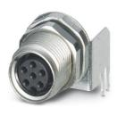
Device connector rear mounting, 6-position, Socket, angled, M8, Rear mounting, M10, Solder pins
