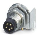
Device connector rear mounting, 5-position, Pin, angled, M8, Rear mounting, M8 x 1, Wave soldering, coding: B - inverse
