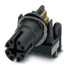
Contact carrier, Ethernet CAT6 $_{\rm A}$  (10 Gbps), 8-position, Socket, angled, M12, coding: X, PCB mounting, Wave soldering, Alternative product in accordance with RoHS II without Exemption 6c (Pb < 0.1 %) item no.: 1237389
