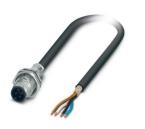
Device connector rear mounting, Universal, 4-position, PUR, black-gray RAL 7021, shielded, Pin, straight, M12-SPEEDCON, coding: A, on free cable end, Rear mounting, M16 x 1.5, Cable connection, cable length: 2 m, PUR halogen-free black, Alternative product in accordance with RoHS II without Exemption 6c (Pb < 0.1 %) item no.: 1239251
