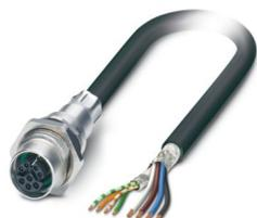
Device connector rear mounting, Ethernet hybrid CAT5 (100 Mbps) CAT5 (100 Mbps), 8-position, Socket, straight, M12-SPEEDCON, coding: Y, on free cable end, Rear mounting, M16 x 1.5, Hybrid cable, cable length: 1 m, Alternative product in accordance with RoHS II without Exemption 6c (Pb < 0.1 %) item no.: 1238750
