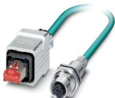
Assembled Ethernet cable, CAT5e, shielded, 2-pair, AWG 26 stranded (7-wire), RAL 5021 (water blue), M12 flush-type socket, rear/screw mounting with M16 thread on RJ45 plug/IP67 push-pull metal housing, line, length 2 m
