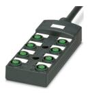
Distributor box, connection method: M12-SPEEDCON-socket Plastic, number of slots: 8, number of positions: 4, coding: A, slot assignment: single, status display: Yes, npn; master cable connection: Fixed connection 180°, PUR/PVC, cable length: 10 m, shielding: no
