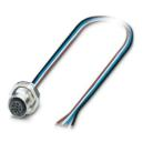
Device connector rear mounting, Universal, 4-position, Socket, straight, M12-Standard, coding: A, on free cable end, Rear mounting, Pg9, Individual wires, cable length: 0.5 m, 0.34 mm<sup>2</sup>, TPE litz wire
