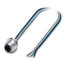
Device connector front mounting, Universal, 4-position, Pin, straight, M12-Standard, coding: A, on free cable end, Front mounting, M16 x 1.5, Individual wires, cable length: 0.5 m, 0.34 mm<sup>2</sup>, TPE litz wire
