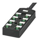
Distributor box, application: Robots and drag chains, connection method: M12-SPEEDCONsocket Metal, number of slots: 8, number of positions: 5, coding: A, slot assignment: Double, status display: Yes, pnp; master cable connection: Fixed connection 180°, PUR, halogen free, highly flexible, highly flexible, cable length: 5 m, shielding: no
