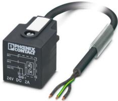
Sensor/actuator cable, 3-position, PUR halogen-free, black-gray RAL 7021, free cable end, on Valve connector A, with 1 LED, Wiring: Freewheeling diode, cable length: 3 m
