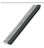
Band ferrules, 1.5 mm<sup>2</sup>, sleeve length 8 mm, with plastic collar, according to DIN 46228-4, color: black, equipped with function end for safe and convenient processing with the Crimphandy, 20 strips with 50 sleeves per strip.
