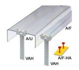
Flat-ribbon cover, for covering terminal strips, 2 mm thick, 5 cm wide, an additional requirement are 2 E/UK end brackets and 2 adjustable VAH cover holders. The max. supply length is 100 cm
