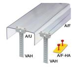
Flat-ribbon cover, for covering terminal strips, 2 mm thick, 2,0 cm wide, an additional requirement are 2 E/UK end brackets and 2 adjustable VAH cover holders. The max. supply length is 100 cm
