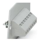
Panel feed-through terminal block, connection method: Screw connection with tension sleeve, Cable lug connection, number of positions: 1, load current: 76 A, cross section: 0.5 mm<sup>2</sup> - 25 mm<sup>2</sup>, connection direction of the conductor to plug-in direction: -90 °, width: 12 mm
