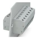
Panel feed-through terminal block, connection method: Screw connection with tension sleeve, Screw connection with tension sleeve, number of positions: 1, load current: 76 A, cross section: 0.5 mm<sup>2</sup> - 25 mm<sup>2</sup>, connection direction of the conductor to plug-in direction: 0 °, width: 12 mm
