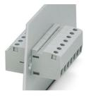
Panel feed-through terminal block, connection method: Screw connection with tension sleeve, Screw connection with tension sleeve, number of positions: 1, load current: 57 A, cross section:  $0.5 \text{ mm}^2$  - 16 mm<sup>2</sup>, connection direction of the conductor to plug-in direction: 0°, width: 10.1 mm
