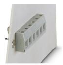
Panel feed-through terminal block, connection method: Screw connection with tension sleeve, Solder connection, number of positions: 1, load current: 32 A, cross section: 0.2 mm<sup>2</sup> - 6 mm<sup>2</sup>, AWG 24 - 10, connection direction of the conductor to plug-in direction: 0 °, width: 10 mm
