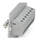
Panel feed-through terminal block, connection method: Screw connection with tension sleeve, Cable lug connection, number of positions: 1, load current: 101 A, cross section: 6 mm<sup>2</sup> - 35 mm<sup>2</sup>, connection direction of the conductor to plug-in direction: 0 °, width: 15 mm
