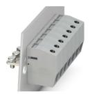
Panel feed-through terminal block, connection method: Screw connection with tension sleeve, Cable lug connection, number of positions: 1, load current: 101 A, cross section:  $6~\text{mm}^2$  - 35 mm², connection direction of the conductor to plug-in direction:  $0~^\circ$ , width: 15 mm
