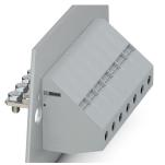
Panel feed-through terminal block, connection method: Screw connection with tension sleeve, Cable lug connection, number of positions: 1, load current: 101 A, cross section: 6 mm² - 35 mm², connection direction of the conductor to plug-in direction: -90 °, width: 15.1 mm, color: gray
