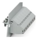
Panel feed-through terminal block, connection method: Screw connection with tension sleeve, Cable lug connection, number of positions: 1, load current: 150 A, cross section:  $16 \text{ mm}^2 - 50 \text{ mm}^2$ , connection direction of the conductor to plug-in direction:  $-90 \, ^\circ$ , width:  $18.8 \, \text{mm}$
