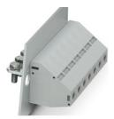
Panel feed-through terminal block, connection method: Screw connection with tension sleeve, Cable lug connection, number of positions: 1, load current: 150 A, cross section:  $16 \text{ mm}^2 - 50 \text{ mm}^2$ , connection direction of the conductor to plug-in direction:  $-90 \, ^\circ$ , width:  $18.8 \, \text{mm}$
