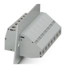
Panel feed-through terminal block, connection method: Screw connection with tension sleeve, Screw connection with tension sleeve, number of positions: 1, load current: 150 A, cross section: 16 mm<sup>2</sup> - 50 mm<sup>2</sup>, connection direction of the conductor to plug-in direction: -90 °, width: 18.8
