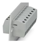
Panel feed-through terminal block, connection method: Screw connection with tension sleeve, Screw connection with tension sleeve, number of positions: 1, load current: 101 A, cross section: 6 mm² - 35 mm², connection direction of the conductor to plug-in direction: 0 °, width: 15.1 mm
