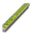
Connection terminal block, nom. voltage: 300 V, nominal current: 125 A, connection method: Screw connection, Rated cross section: 35 mm², cross section: 2.5 mm² - 35 mm², mounting: Neutral busbar, color: green-yellow
